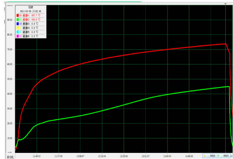
Real-time temperature curve of furnace and plate backing (Green: plate backing, Red: furnace )
