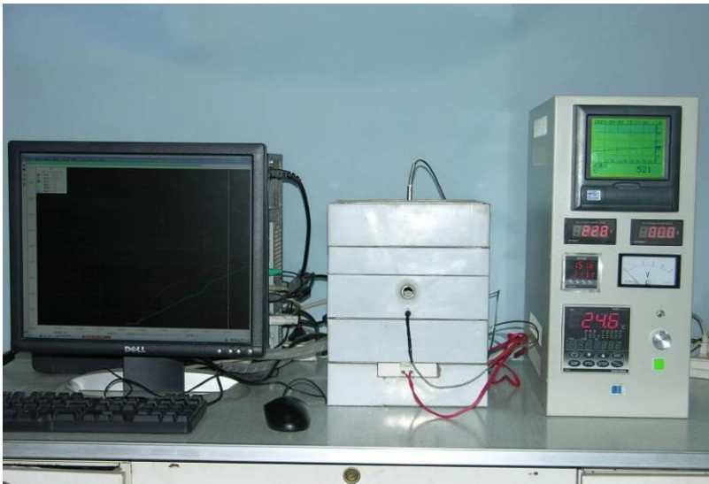
Fire-proof Performance of Coating Quick-Test Equipment
